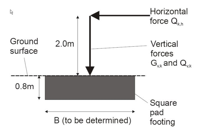
Permanent: Vertical  $G_{v,k} = 1000 \text{ kN}$ , excluding weight of foundation
